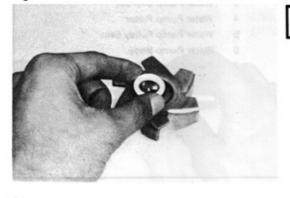
Install seal and cover on rotor.
