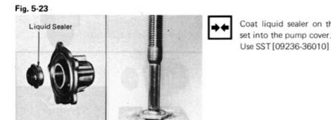
Coat liquid sealer on the seal set, and press seal set into the pump cover. Use SST [09236-36010]
