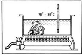
Heat the water pump cover up to around  $75^{\circ}$  to  $85^{\circ}\text{C}$  (167° to 185°F).
