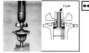
Using a press, force in rotor.
