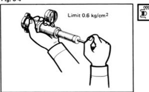
Using the cap tester, measure the valve opening pressure. If lower than the limit, replace cap.
