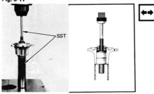
Using SST [09236-36010] and a press, force out the bearing from the pump cover.
