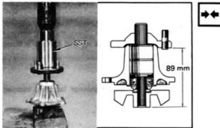
Using a press and SST[09238-40010], force in the pulley seat.
